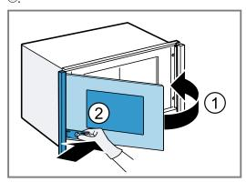
There may be noises when the panels are removed. Take hold of the panel on the side without the door hinges using both hands and remove it.
