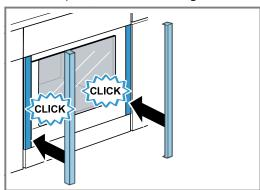
The groove on the fascia panels must be at the top. Position the groove on the panels above the corresponding transverse rib on the red fastening part.
