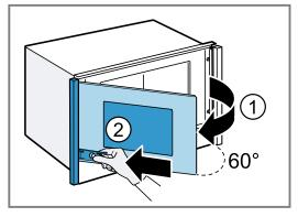
2. To loosen the panel, close the appliance door ① and at the same time press the fastening element on the appliance door down and towards the panel
